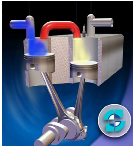
Split-cycle engine divides 4-stroke operation into separate cylinders.
